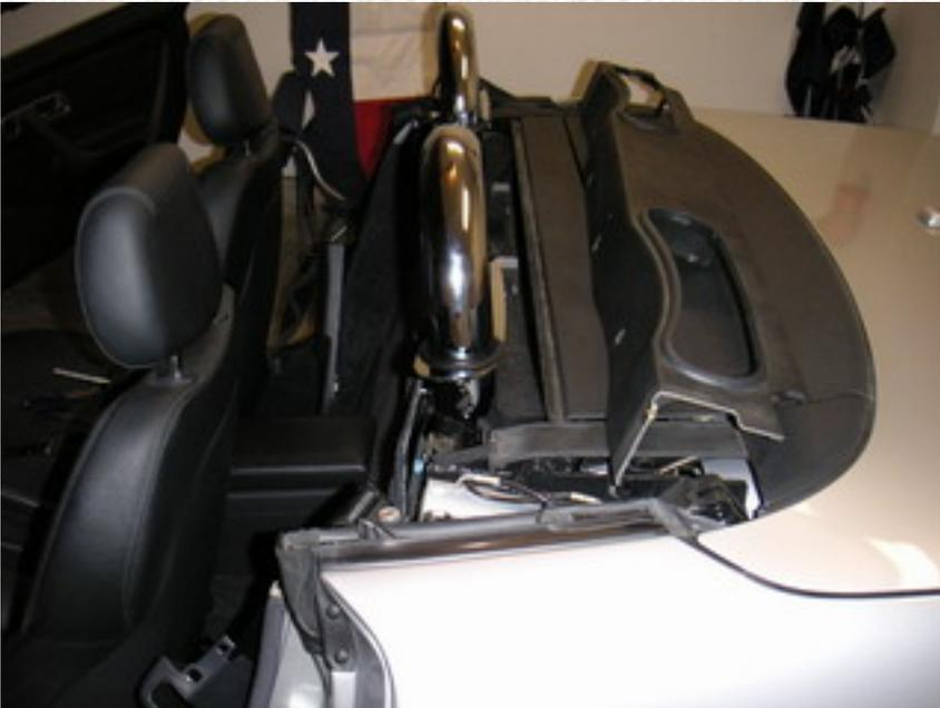
As soon as we know that the bars do not break the rear window, let's tighten the roll bar bolts with full power. Notice that the chrome bars will be leaning slightly forward, like the stock bars.
