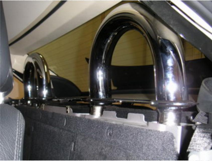
The reason why we do not want to have the bar bolts very tight yet is that it is a good idea to verify that they do not touch to the rear window. Close the top carefully, and make sure there is a gap between the bars and the window.
