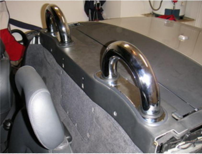
Push the liner (and plates) down, and snap it to the hook in the middle.
