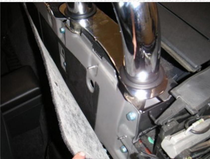
Put the bolts to their places, lift the roll bar as up, as much as possible. Fasten the bolts, but not with full power.
