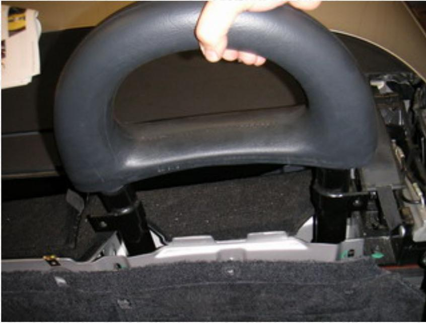
Lift the roll bar up to remove it.
