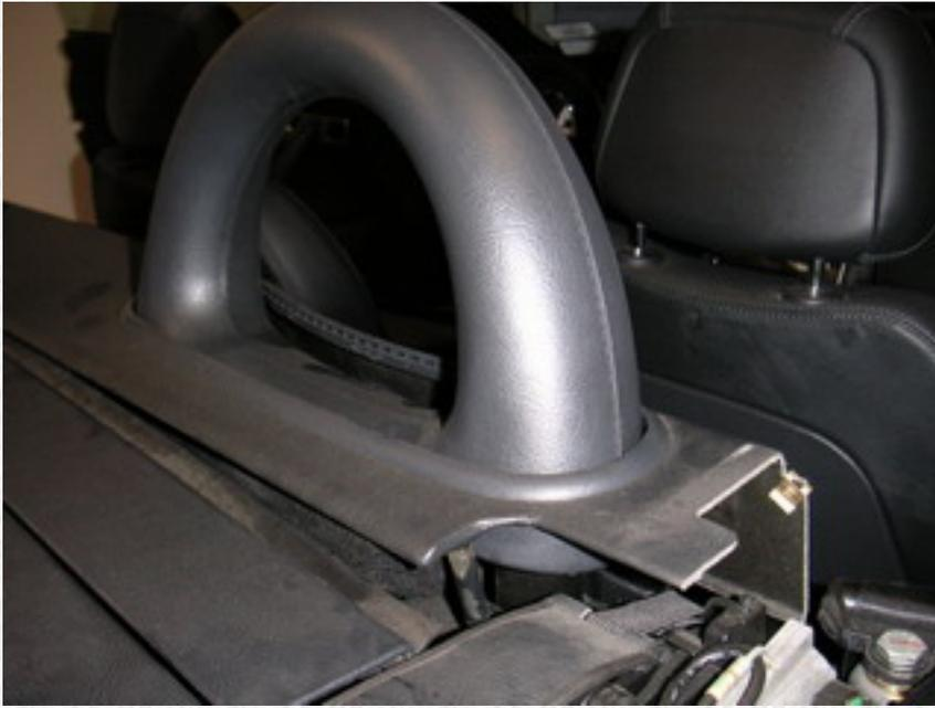
Now we are ready to remove the liner around the roll bars.
