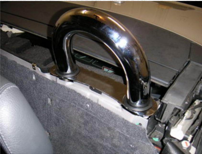
As soon as we have the seals in place, lift the plate as high as possible. This will be useful later on. And let's place the chrome roll bars to the holes where we took the stock bars.
